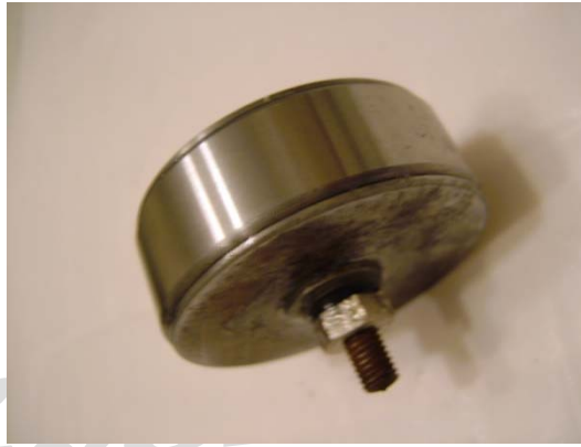
Fig 1: A bearing outer race prepared for plating
